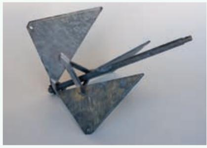
**Devil's fork:** This two-piece Bulwagga faltered in the short scope test, but with 7:1 scope it held fast at 480 pounds.
